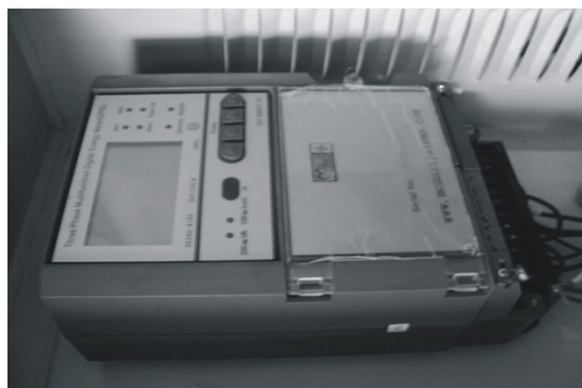
Figure 5. A maximum demand meter. Source: Adenikinju & Oluwayemisi, 2011.
