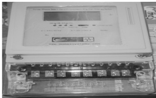
Figure 4. A three-phase smart card prepayment digital energy meter. Source: Adenikinju & Oluwayemisi, 2011.
