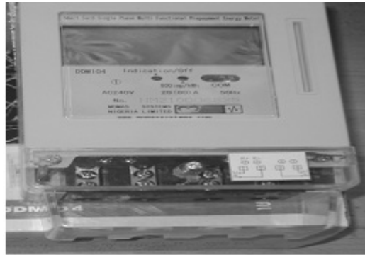
Figure 3. A single-phase smart card digital energy meter. Source: Adenikinju & Oluwayemisi, 2011.
