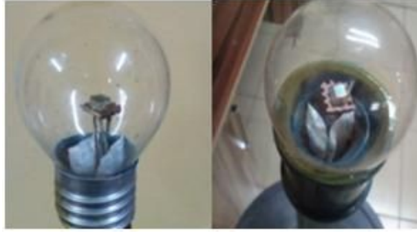
Figure 2 The photodiode enclosed in an evacuated electric bulb
