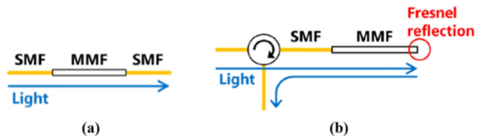
Fig. 6 Conceptual set-ups of a transmissive configuration and b reflectometric configuration. MMF, multimode fiber; SMF, single-mode fiber [67]
